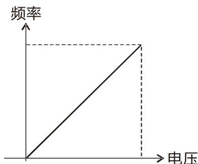
$$F_{\text{command}} = [(ay = \text{bias}) * \text{gain}] * \frac{F_{\text{max}}(01-00)}{10\text{V or } 16\text{mA or } 20\text{mA}}$$
