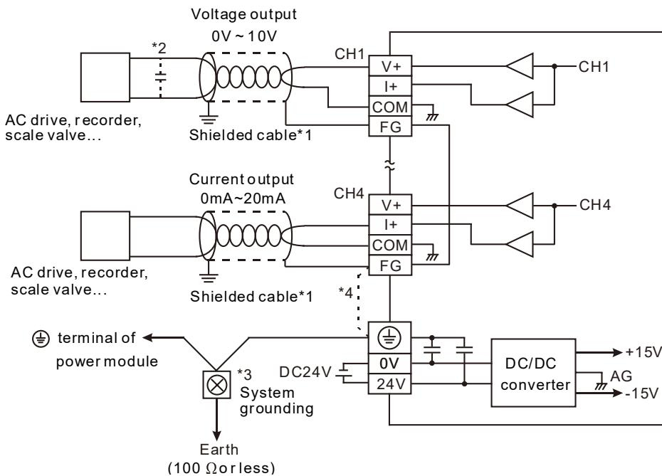
Note 1: When performing analog output, please isolate other power wirings.
